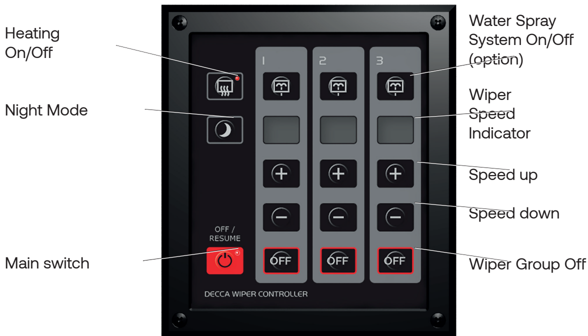
Figure 25 - Wiper Control Panel
