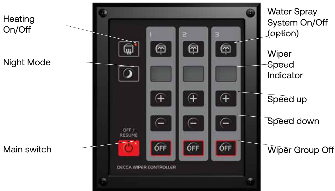
Figure 25 - Wiper Control Panel
